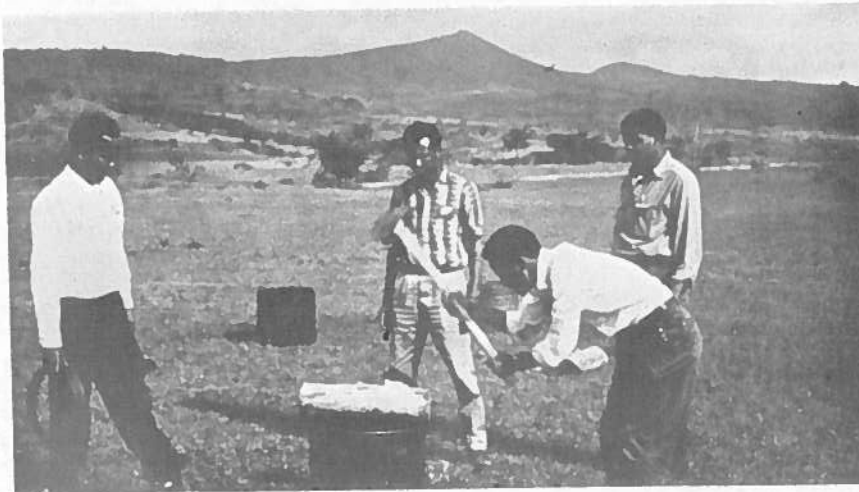
Figure IV-2 - Ethiopian land classification crew prepares for infiltration rate measurement by sinking test cylinder in ground.
